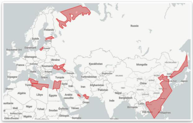
Figure 4-7: Areas at risk of GNSS interference. Source: M-CERT.
